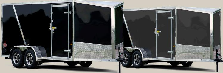
SUPER LOCK... Screwless Exterior Aluminum system is unique to AmeraLite... No other manufacturer has it -or anything like it. SUPER LOCK... Lasts longer, looks much better, wont rust. The inter-locking aluminum panels are glued **and** mechanically fastened so that it doesn't show on the outside.
