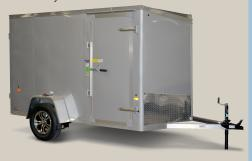
5', 6' and 7' wide models have a rear barn door standard. 8.5' wides comes with ramp door standard. All doors have double automotive bulb seals -locks out dust, moisture, and road grime for superior protection over single weather strip.
