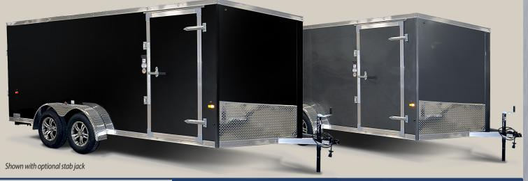
SUPER LOCK™ Screwless Exterior Aluminum system is unique to AmeraLite... No other manufacturer has it -or anything like it. SUPER LOCK... Lasts longer, looks much better, won't rust. The inter-locking aluminum panels are glued and mechanically fastened so that it doesn't show on the outside.
