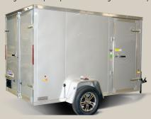
All models have DryMax... Engineered Flooring and walls, standard. These high performance, engineered panels resist moisture and chemicals -will not absorb moisture, swell, warp or delaminate. Stronger and stiffer than plywood.
